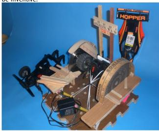
An RC car rear end converted to table saw and disc sander.
